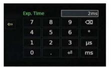
The Exposure time menu allows the camera's exposure to be entered in microseconds, milliseconds or degrees
