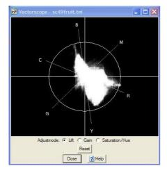
The vector scope displays the image in a color space. The image data is displayed as a three dimensional histogram.
