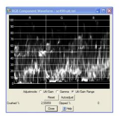
The RGB Wave form displays the wave form for each color separately.
