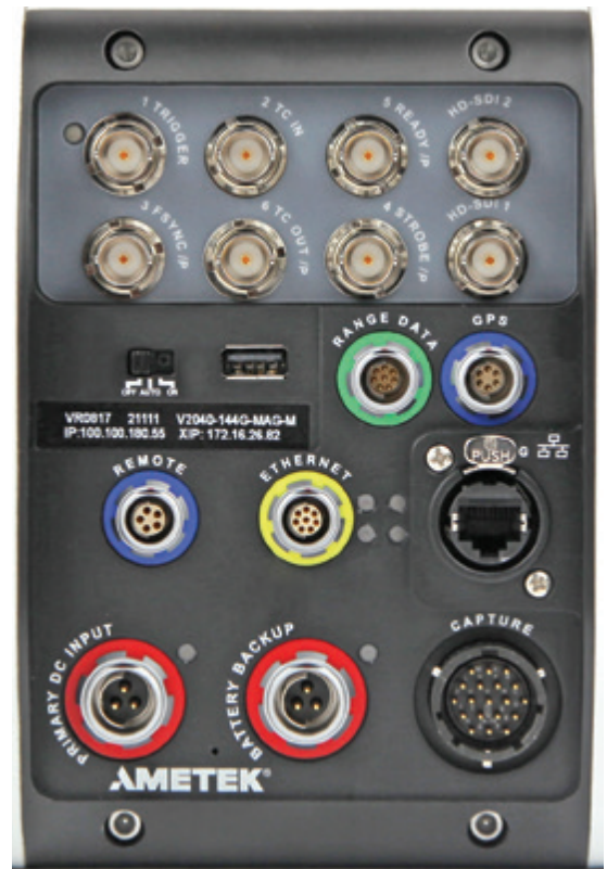
Phantom v2640 - Back Panel
