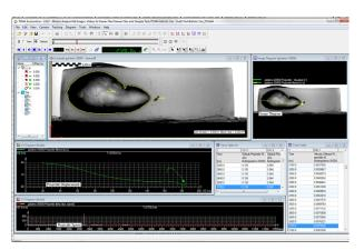
TEMA is used to calculate the rotational volume of the cavity created by the bullet fired into the gelatine. Other parameters such as speed, acceleration, bullet orientation are also analysed.
