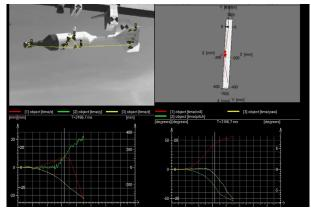
You can use the TEMA Defence software suite to properly calculate the x, y, z coordinates of the object as well as roll, pitch and yaw. The result is presented in grahps and numerical tables.
