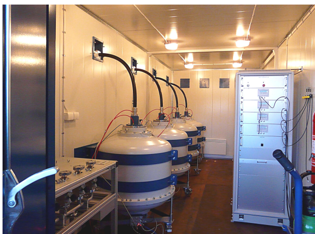
Fig. 20 Containerised flash x-ray system
