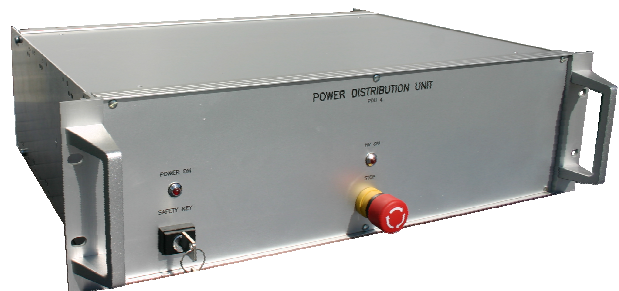
Fig. 3 Model PDU 4 power distribution unit
