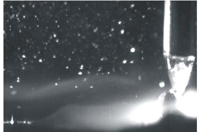
PIV arc welding (2000 fps)
